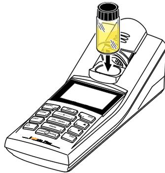
**Inserting a 16 mm cell**
